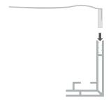
Place the textile print in the frame. Start with the corners and press the silicone strip in the channel.
