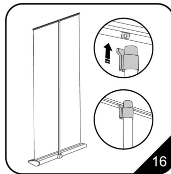
16. The plastic holder at the top of pole slips into the rear slot of the banner beam. A marker on the beam indicates the beam's centre where the pole should be inserted.
